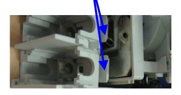
Remove the internal sub assembly from the base and cut the electrical wires to remove the printed circuit boards from the sub assembly
